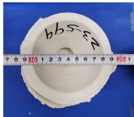
图 4 添加细化剂的型壳面层示意图 Fig.4 Diagram for surface layer of mold shell added with refiner
