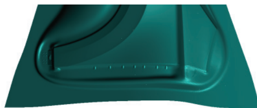
图5 翼子板带水滴补充工艺面 Fig.5 Fender drawing addendum with water-drop shape
