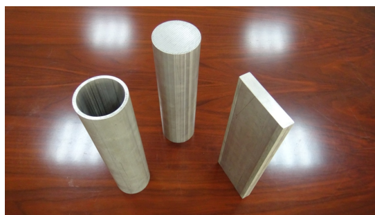
图2 高强铝合金棒材、管材和板带材 Fig.2 High-strength aluminum alloy bar, tube and strip
