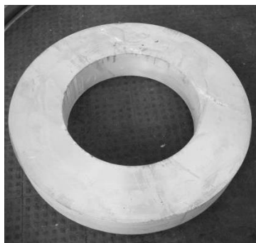
图2 轧制试验坯料 Fig.2 Blank of rolling process
