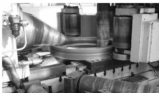
图4 环件轧制过程 Fig.4 Rolling process of annulus
