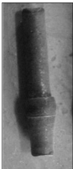
图 3 粗锻台阶/纵向弯曲 Fig. 3 Step/bend flaw in the first upsetting
