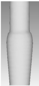
图 13 13^{\circ} 粗镦模拟结果 Fig. 13 The result of simulation in the first upsetting with the cone angle of 13^{\circ}
