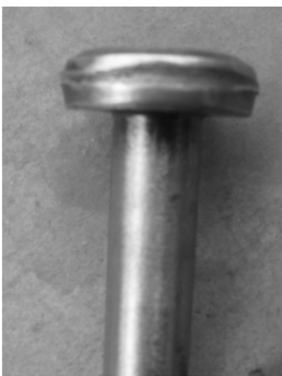
图 12 精镦折叠 Fig. 12 Fold in the last upsetting
