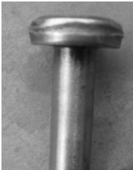
图 4 精锻后的折叠 Fig. 4 Fold in the last upsetting
